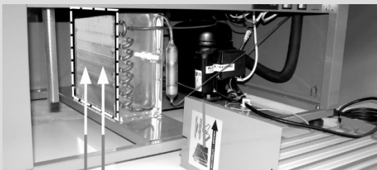
CLEAN THE CONDENSER WITH A VECUUM CLEANER HERE
